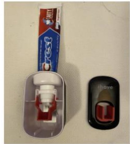
Figure 6: Image of the red lever inserted into the dispenser box. Toothpaste tube is inserted in the top of the device. The front cover with track attached to it rests next to the box.
