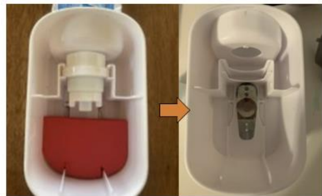
Figure 2: Feedback and toothpaste control evolution. The left box shows mini-cell foam on the back of the device. And the right box shows a bent piece of metal at the back of the device which provides tactile and audio feedback.
