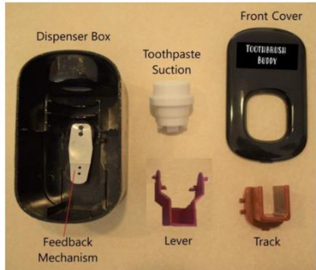
Figure 4: All the parts of the Toothbrush Buddy disassembled and labeled. Depicted: the black Dispenser Box with the metallic Feedback Mechanism inside it, white Toothpaste Suction, grey Lever, black Front Cover, and a red Track.
