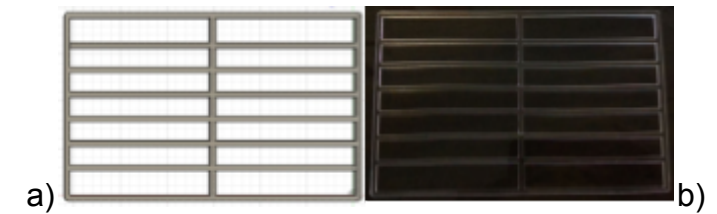
Figure 6. Table template with two columns and seven rows. a) 3D design. b) Final product.
