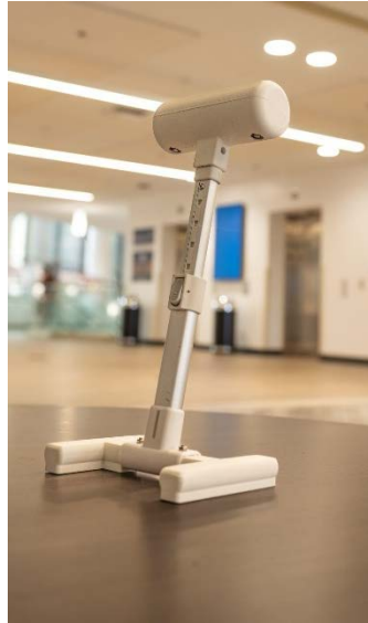
Figure 2: Second iteration of the device with cylindrical 3d printed bar
