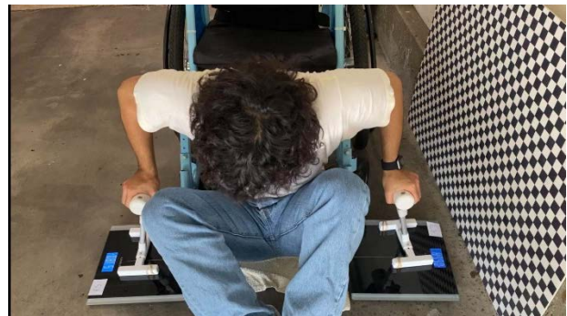
Figure 9A: Rear transfer weight distribution testing with the Assist Handle
