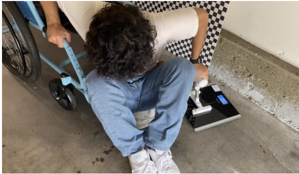
Figure 8A: Sideways transfer weight distribution testing with the Assist Handle
