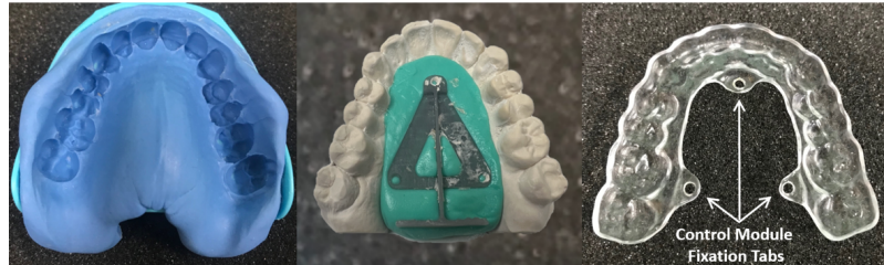
Figure 6. Dental putty impression of the upper teeth (left panel). Dental stone model with the fixation tab preform on a base of putty (middle panel). The finished guard has 3 precisely drilled holes in the fixation tabs that line up with the male stems on the control module (right panel).
