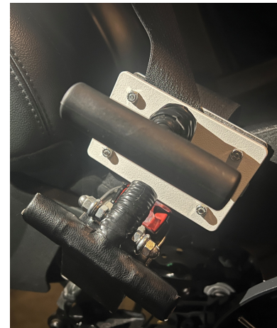
Figure 3. Buckle and receiver unit together with belt buckled.
